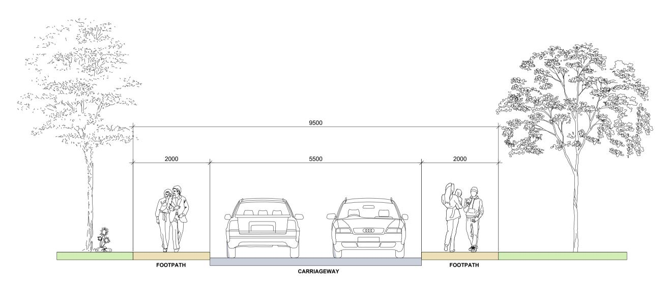
TYPICAL CROSS SECTION B: TYPICAL INTERNAL STREET
